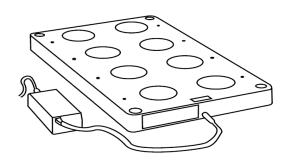
The INDIVIDUAL DIRECT MINI CHARGER charges one single lamp and operates with the following adapter: Input 100-240V AC  $^{\sim}$  50/60 Hz - Output DC 6V 1A
